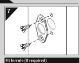
Timber windows may require a ferrule. Mark ferrule fixing holes by placing ferrule centrally over bolt hole. Drill two 2.5mm pilot holes and screw ferrule into place.
