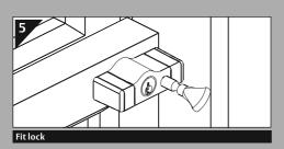
Fit lock body to window using standard screws. If lock operates correctly once bolt is fitted, replace standard screws with one way screws for greater security.
