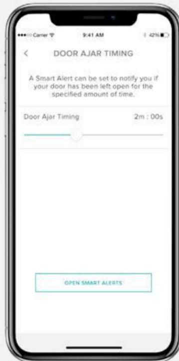
1. The first step in setting up Door Ajar notifications is to set Door Ajar Timing. The time increment selected determines how long your door can be open before you are alerted.
