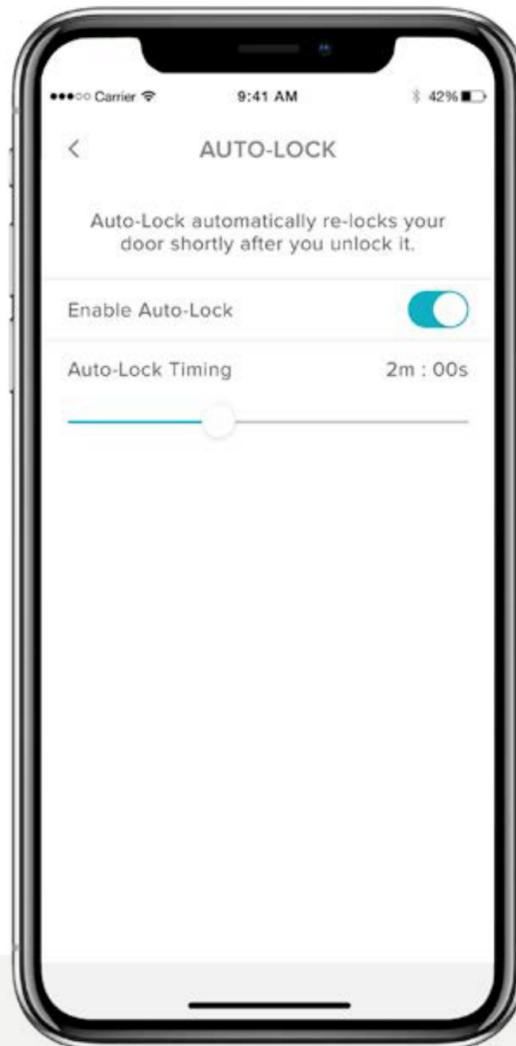
**Auto-lock means you can automatically lock itself after a specified time period. Now, with the included DoorSense™ technology, which informs you whether your door is open or closed, you can program your Smart Lock to lock automatically as soon as it detects that your door is closed.**
